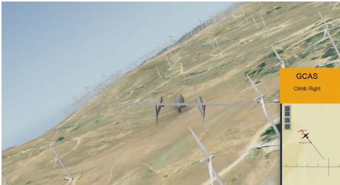
Figure 2.4.3-1: Screen grab from the National Aeronautics and Space Administration (NASA) video showing a controlled Expandable Variable Autonomy Architecture (EVAA) Ground Collision Avoidance (GCAS) terrain avoidance maneuver, simulated by a HQ-90 UAS, flown by a NASA pilot for the DoD live demonstration ( NASA https://www.nasa.gov/sites/default/files/styles/side_image/public/thumbnails/image/resilient_autonomy_image.png?itok=kDNm5zTL ) [7].
