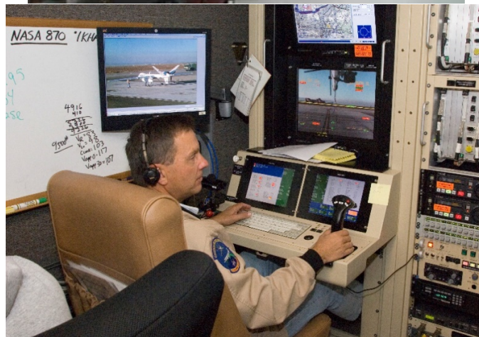
Figure 2.1.2-1: (above left) an early-model General Atomics (GA-ASI) (General Atomics Aeronautical Systems Inc.) (Poway, California, U.S.A.) mobile Ground Control Station (GCS) ( NASA https://www.nasa.gov/sites/default/files/images/171917main_mobile_330.jpg ); and Figure 2.1.2-2: (above right) the pilot-in-command console inside the National Aeronautics and Space Administration (NASA) Ikhana Ground Control Station (GCS) (NASA photo ED07-0243-18).
