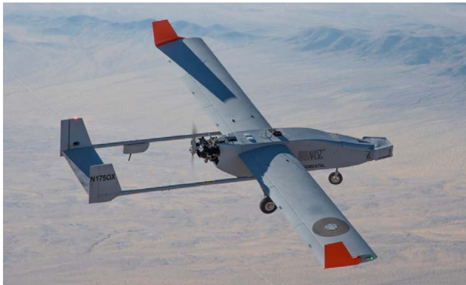
Figure 2.3.1-1: The Navmar Applied Sciences Corporation (NASC) RQ-23 TigerShark XP™ UAS in flight during Flight Test 6 (NASA photo AFRC2019-0142-10).
